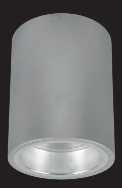
Surface mounted downlight for metal halide lamp. Body is made of aluminium (standard white – available in any RAL colour on request). Reflector is made of aluminium – sandblasted.
